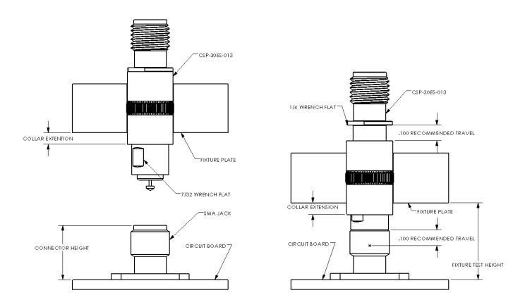
4) The 7/32" or 1/4" wrench flats may be used to connect the SMA interface cable
