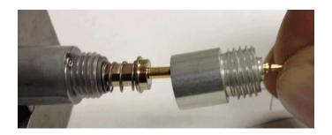
3.2.5: Apply a small amount of Loctite 220 or 242 to threads on gear motor, then thread housing onto gear motor until finger tight as shown below.
