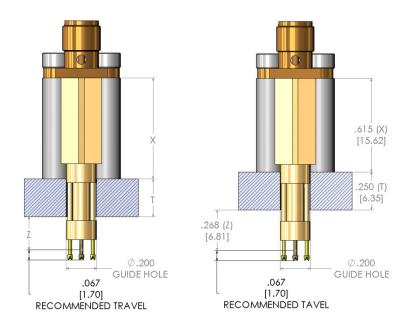
3) Drill THRU hole with a diameter of .200" (5.08mm) into test fixture. This hole is used to align the coax.
