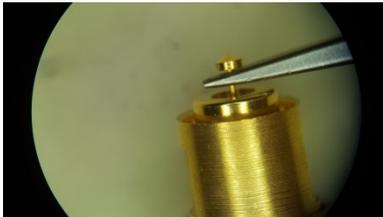
**Pull under probe head with tweezers.**
