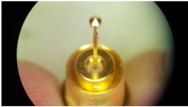
Insert new signal probe, barrel side first.
