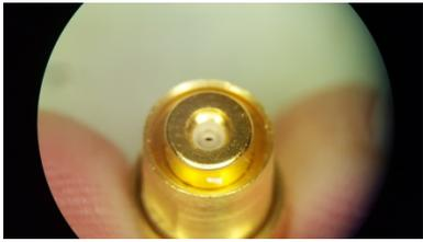
Under microscope, locate the hole in the plastic Insulator.
