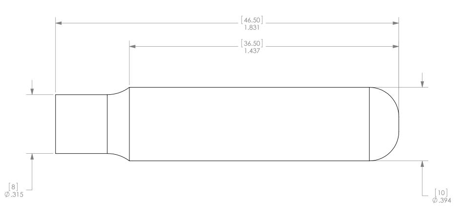
UNLESS OTHERWISE SPECIFIED, DIMENSIONS ARE IN INCHES. **TOLERANCES ARE:** dr .X = +/-.06 ANGLES = +/- 2° .XX = +/-.03chk .XXX = +/-.005.XXXX = +/-.0005app TAPER ON ANY DIA. .002/IN MAX
